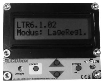
The LCDbox is connected via a 6-pole wire lead to LTR6. The black marking of the connector faces the middle of LCDbox; on the LTR6 the black marking faces the bottom.
